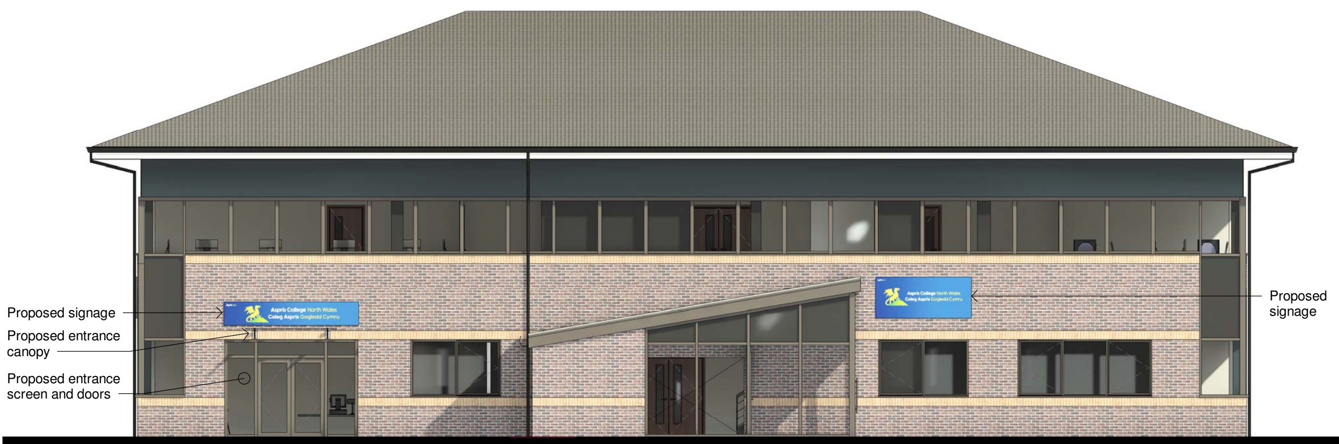
1 Proposed South East Elevation 1 : 100
