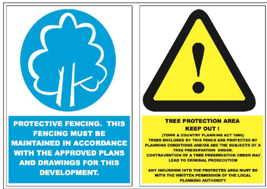
Protective Barrier Fencing - Example Design
