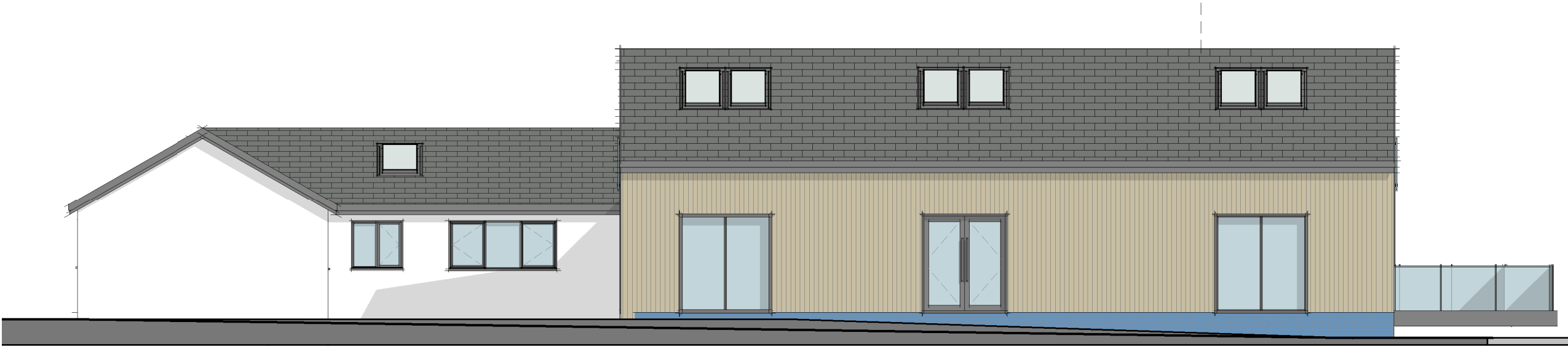
Proposed - Rear Elevation Scale: 1 : 100
