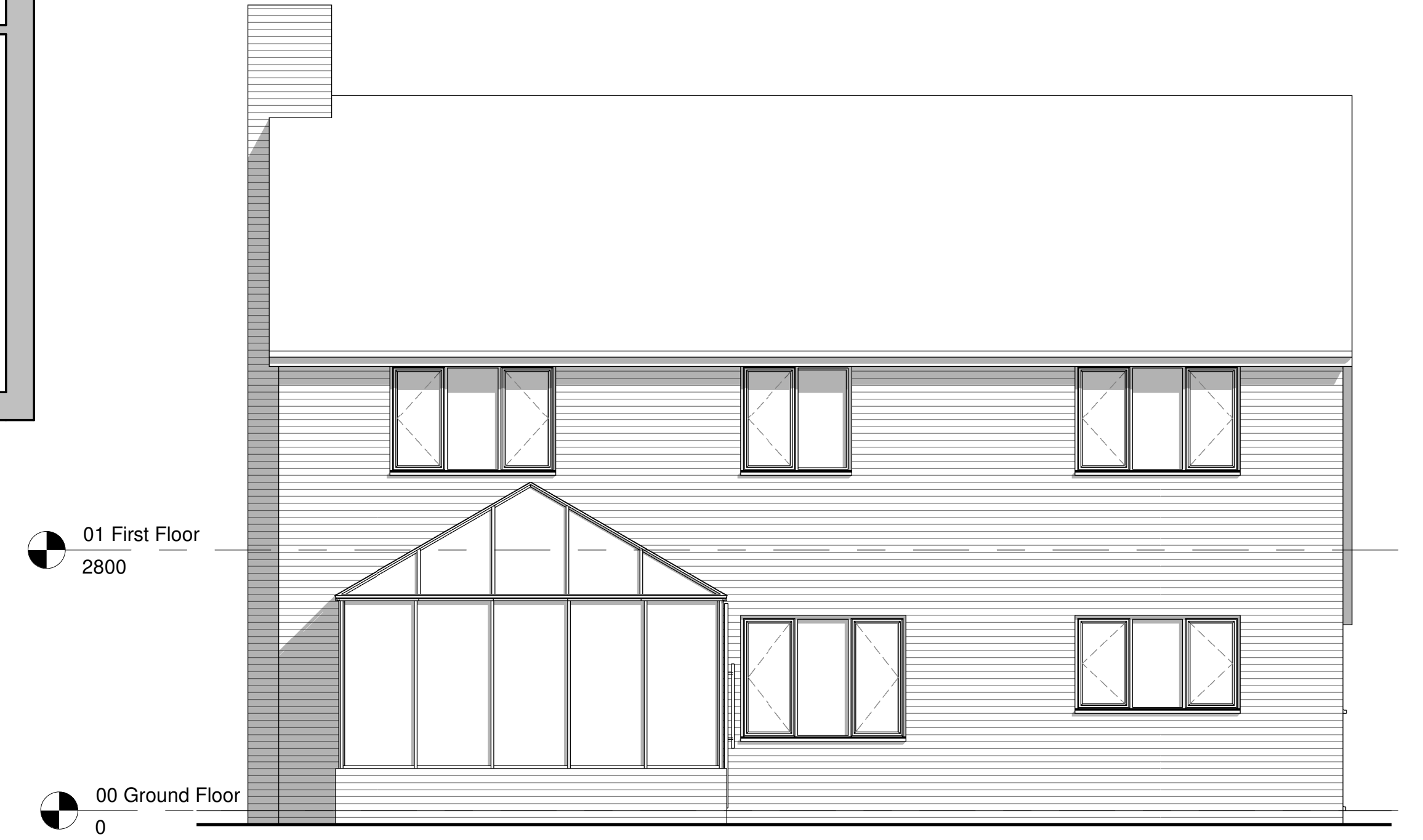
Existing South East Elevation 1 : 50
