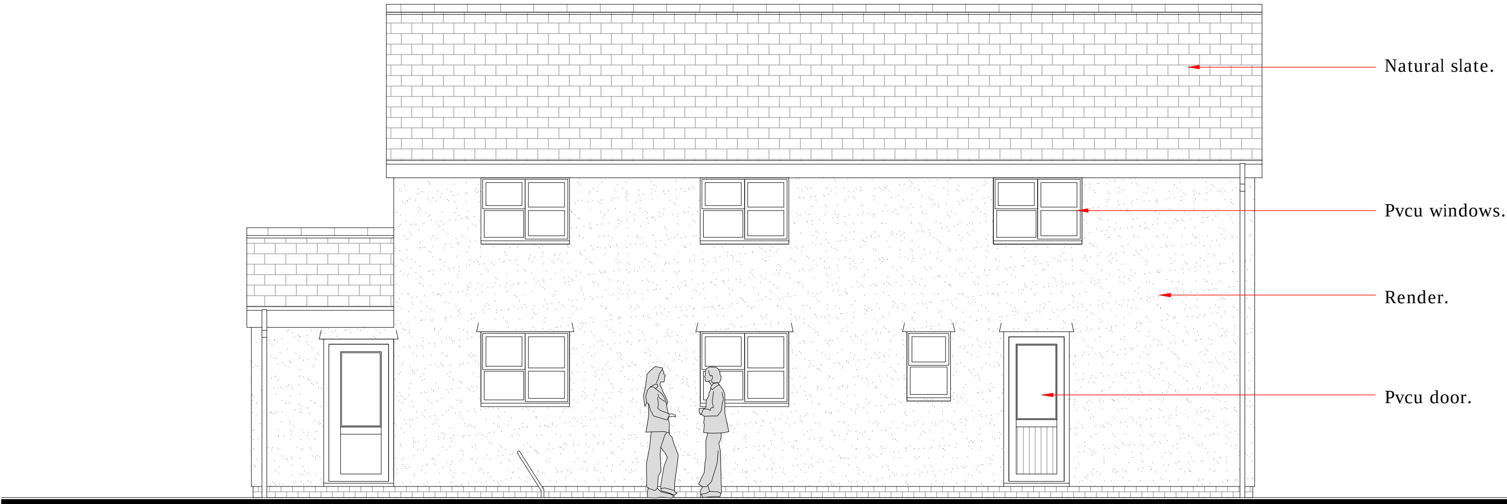
Existing Front Elevation 1:100
