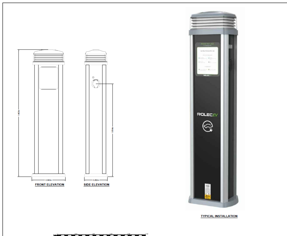
Figure 3.2: Electric Vehicle Charging Point Details
