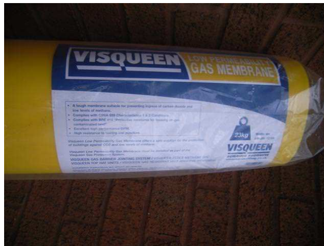
Photograph 17: If no product labels are present then inspect stores for product types. Note membrane shown is not specific for radon protection on this site and is only used as an example.
