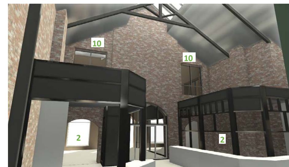
3D view of retained/refurbished historic units 1 & 24. Highlighting opportunity to extend both units through to units 10A and 10 behind. Also opportunity to form glazed first floor openings, providing views between the butchers market and new first floor unit
