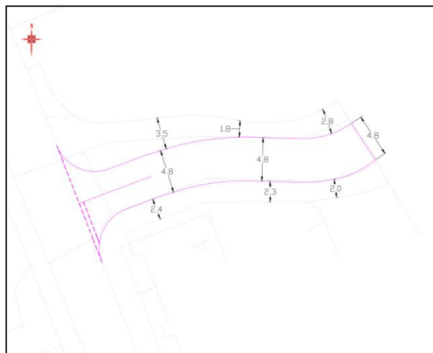
Figure 14: Proposed Upgrades to Existing Shared Access Road
