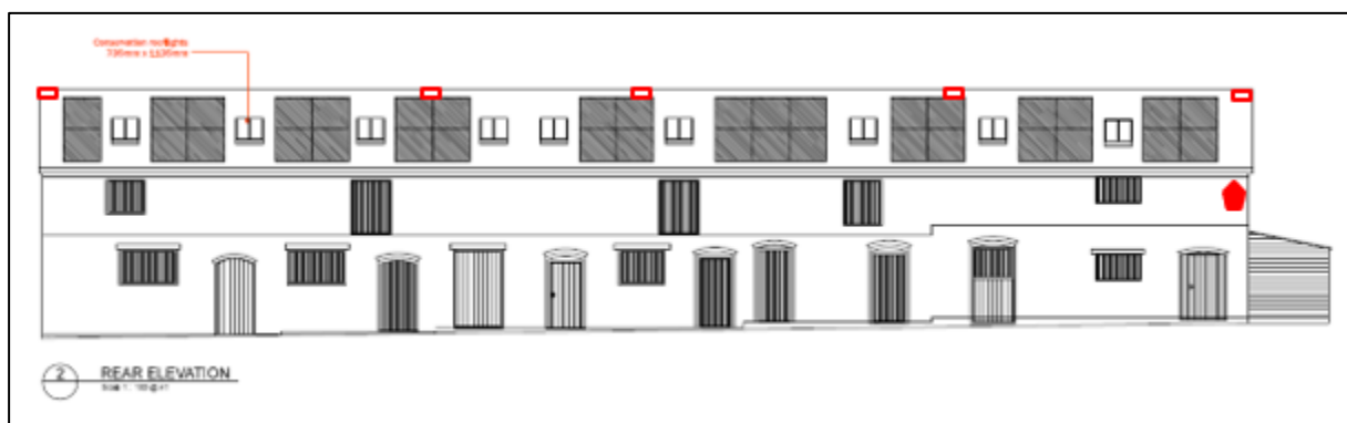
Figure 13. Locations of Beaumaris bat box, or equivalent, (red pentagon) and lifted ridge tiles (red rectangles) on converted Barn. South facing windows will have vertical wooden slats reducing light spill along this elevation.
