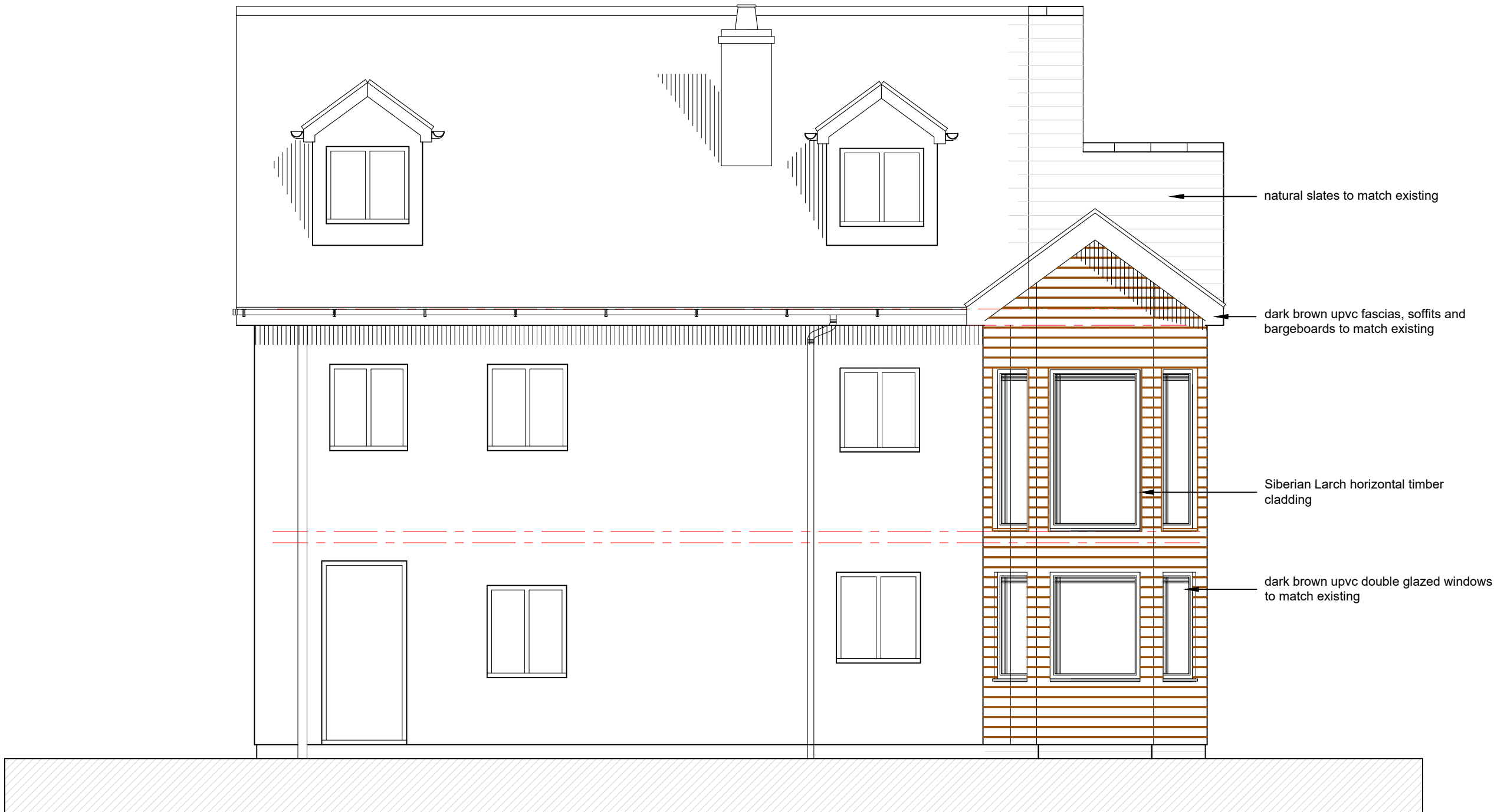
FRONT (SOUTH WEST) ELEVATION
