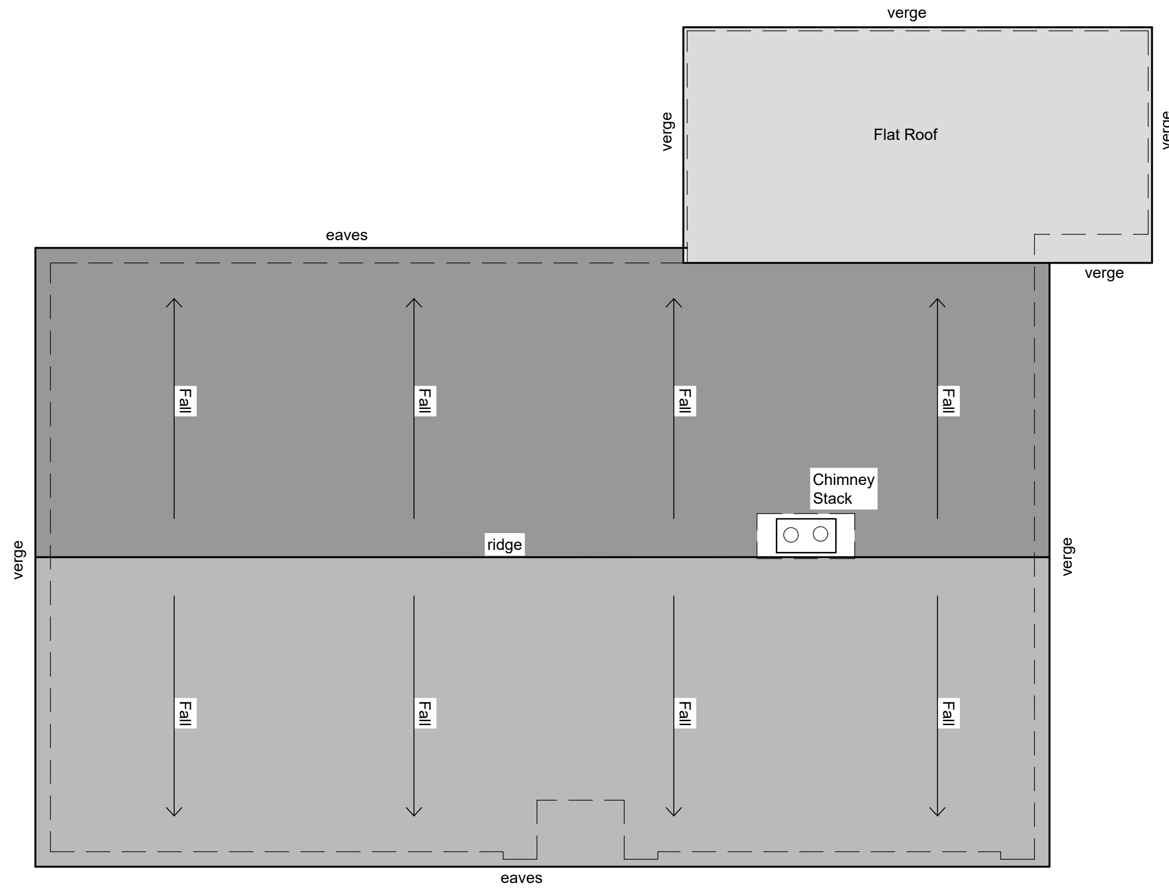
EXISTING ROOF PLAN 1:50
