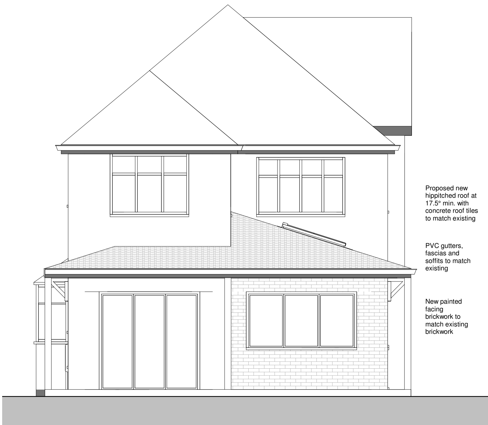
Proposed Rear Elevation
