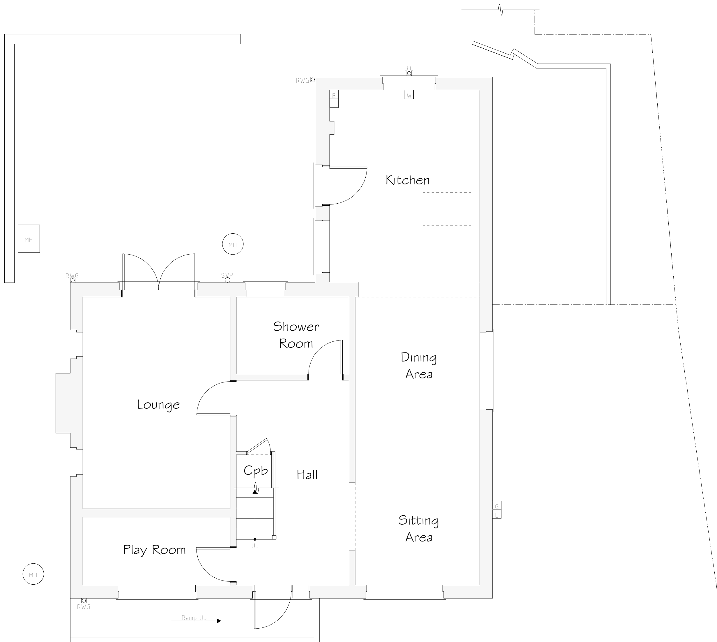
Ground Floor Plan 1:50
