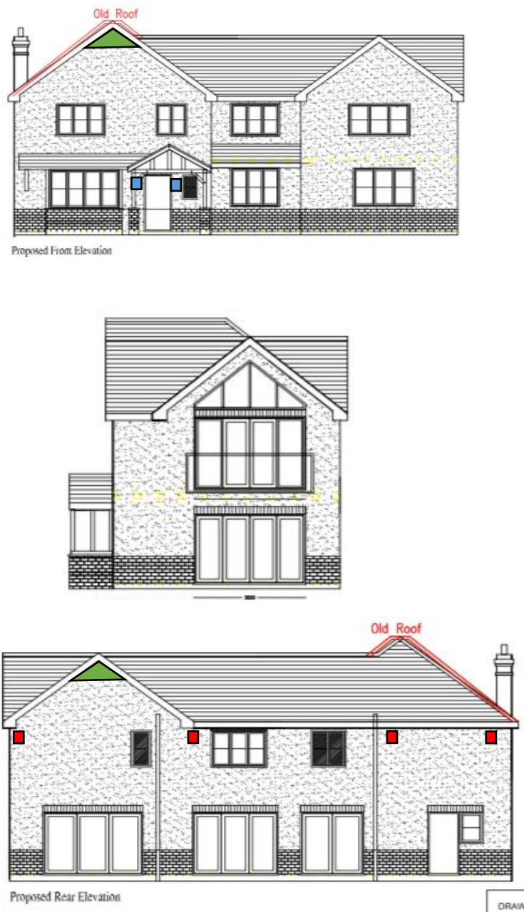
Figure 7: Annotated site plans for the location the bird nesting features. Bird boxes are shown by the red shapes and eaves/ridge overhangs are shown by the green shapes. Please note – the annotations on this image are not to scale.
