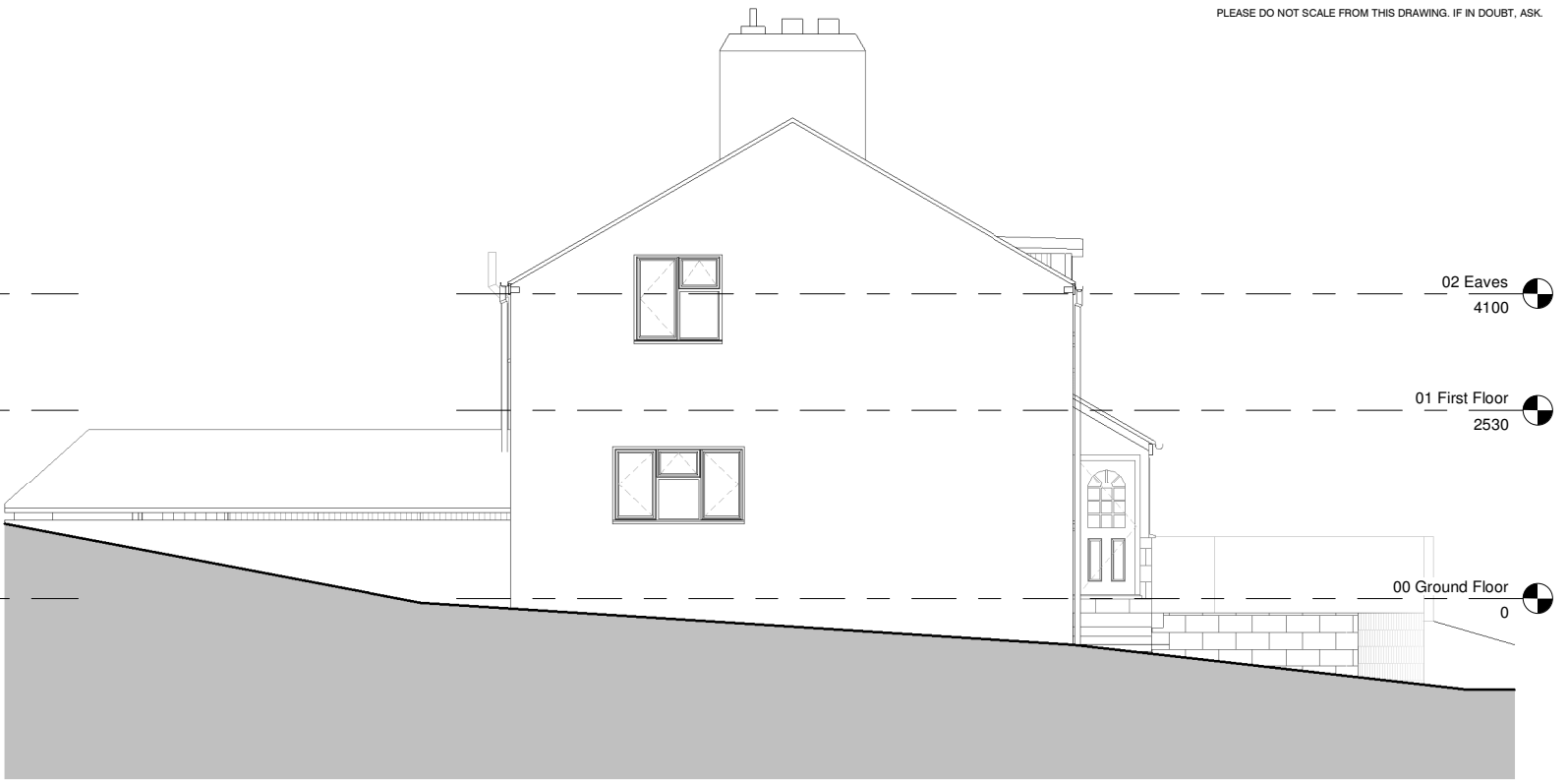
Existing West Elevation 1 : 50
