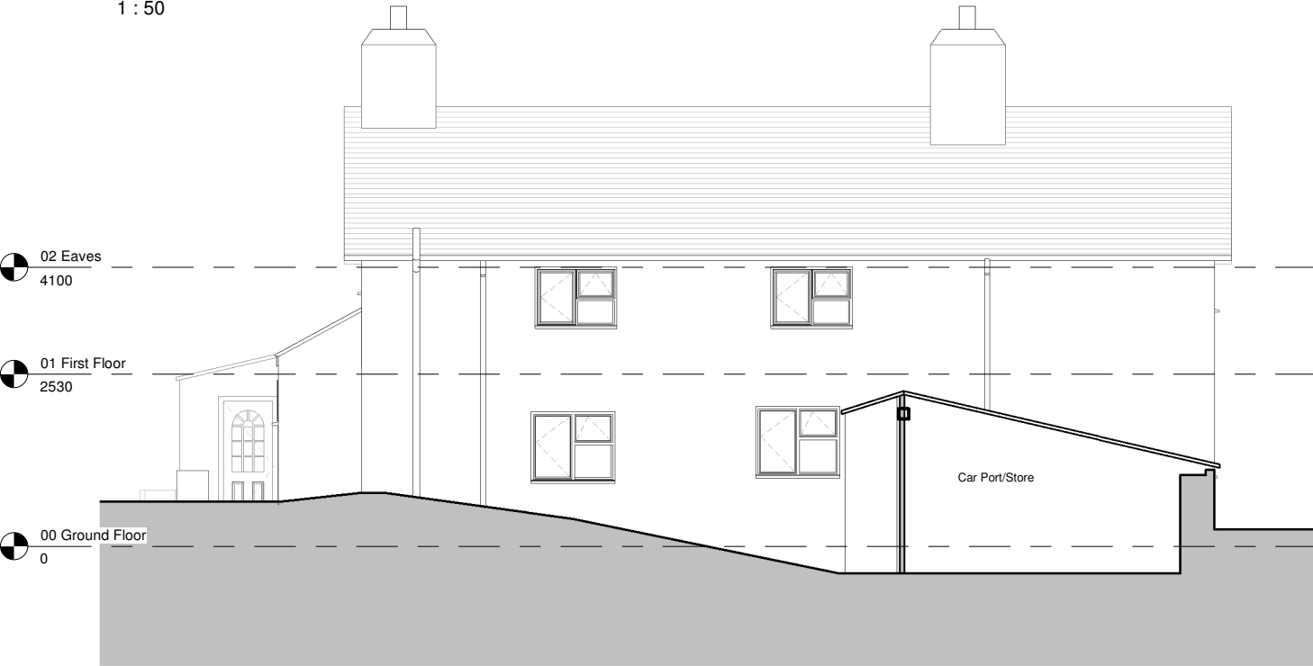
Existing North Elevation 1 : 50
