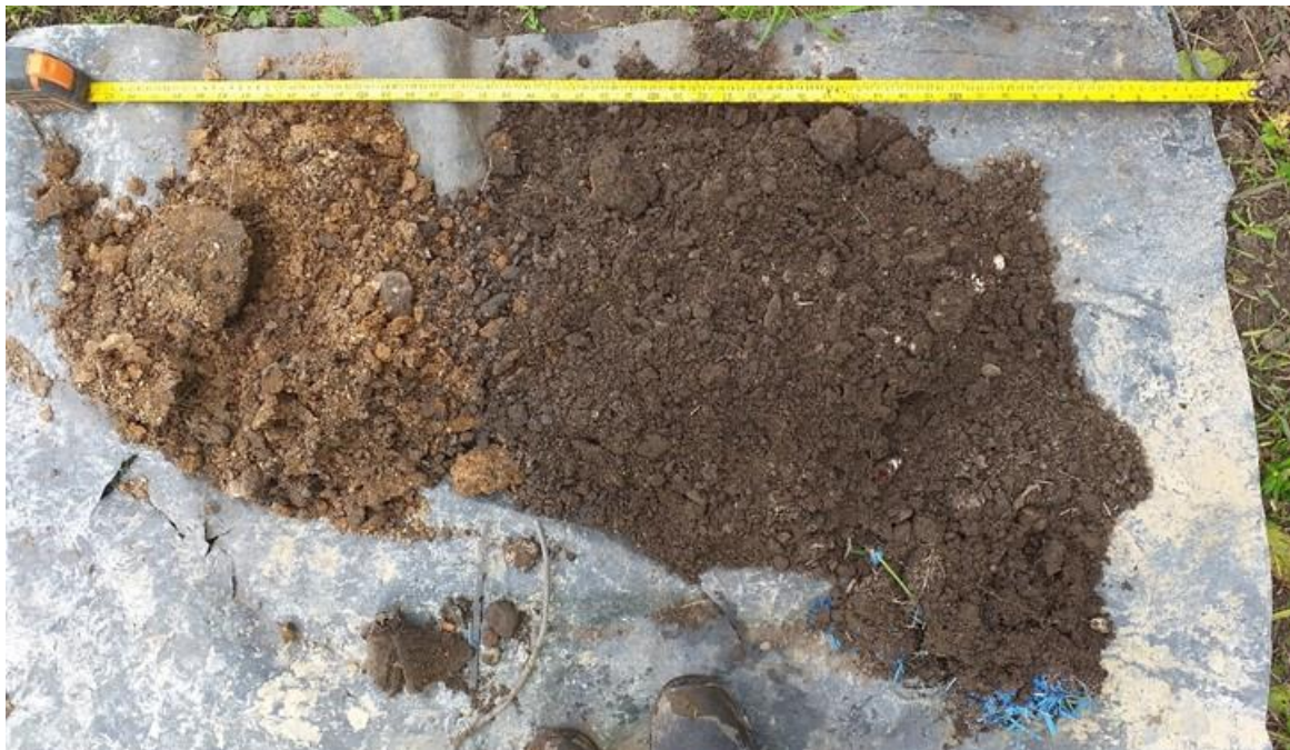
Photo 14: HP08 arisings recovered from 0 to 0.63mbgl. Depth below ground increases from right to left of image.
