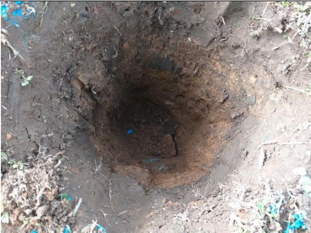
Photo 24: HP13 orangish brown natural material visible below shallow (0.08 to 0.2mblg) made ground.
