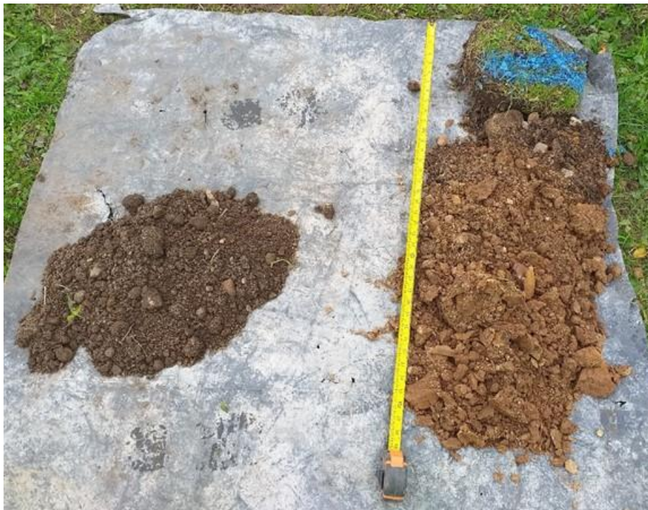
Photo 16: HP09 arisings recovered from 0 to 0.53mbgl. Depth below ground increases from top to bottom of image.
