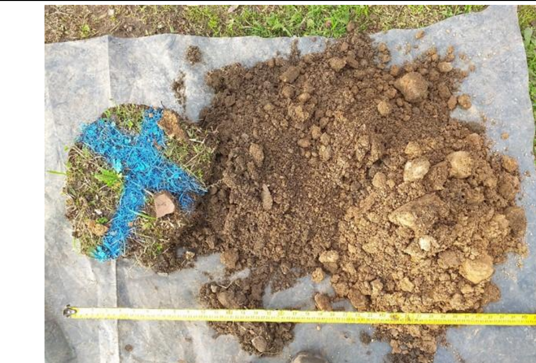
Photo 30: HP18 arisings recovered from 0 to 0.6mbgl. Depth below ground increases from left to right of image.
