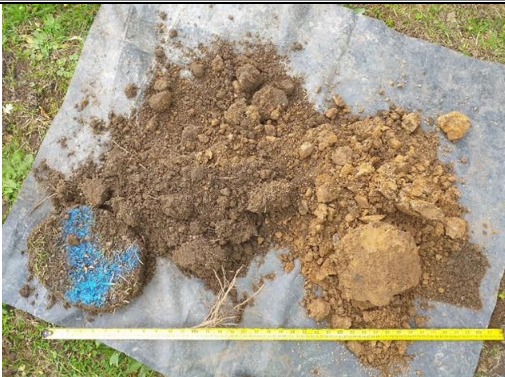
Photo 20: HP11 arisings recovered from 0 to 0.5mbgl. Depth below ground increases from left to right of image.
