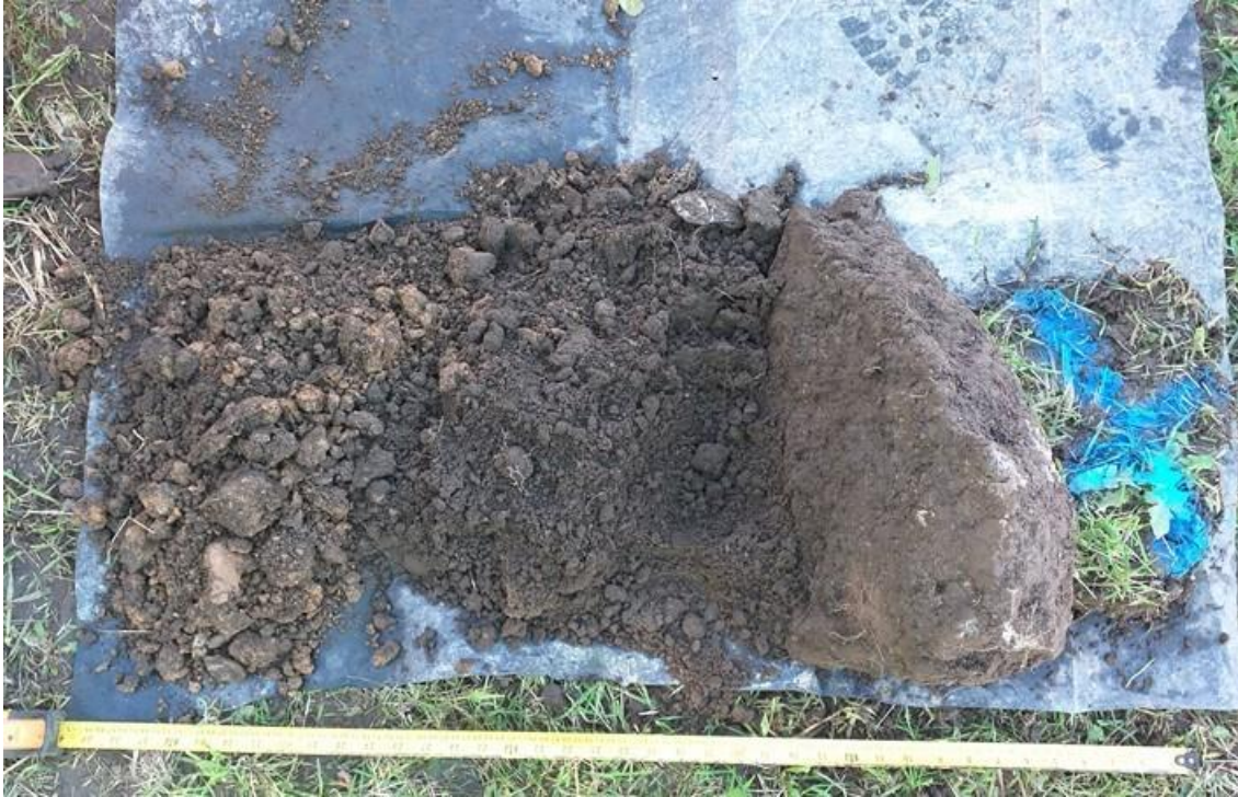
Photo 1: HP01 arisings recovered from 0 to 0.55mbgl. Depth below ground increases from right to left of image.
