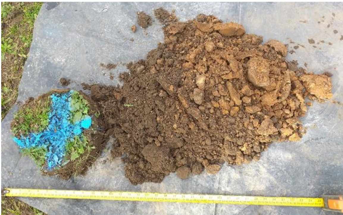
Photo 22: HP12 arisings recovered from 0 to 0.4mbgl. Depth below ground increases from left to right of image.
