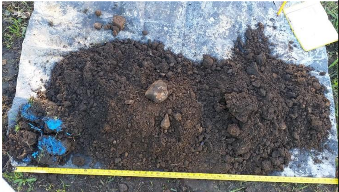
Photo 4: HP03 recovered arisings from 0 to 0.8m bgl. Depth below ground increases from left to right of image.
