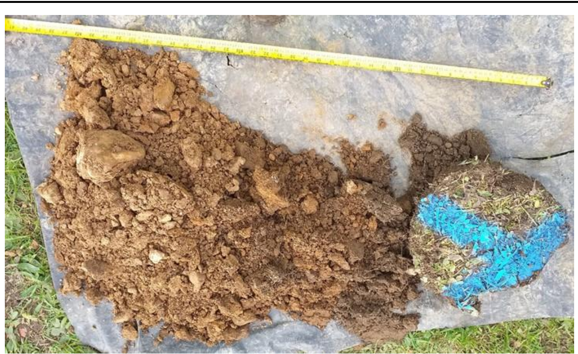
Photo 29: HP17 arisings recovered from 0 to 0.6mbgl. Depth below ground increases from right to left of image.
