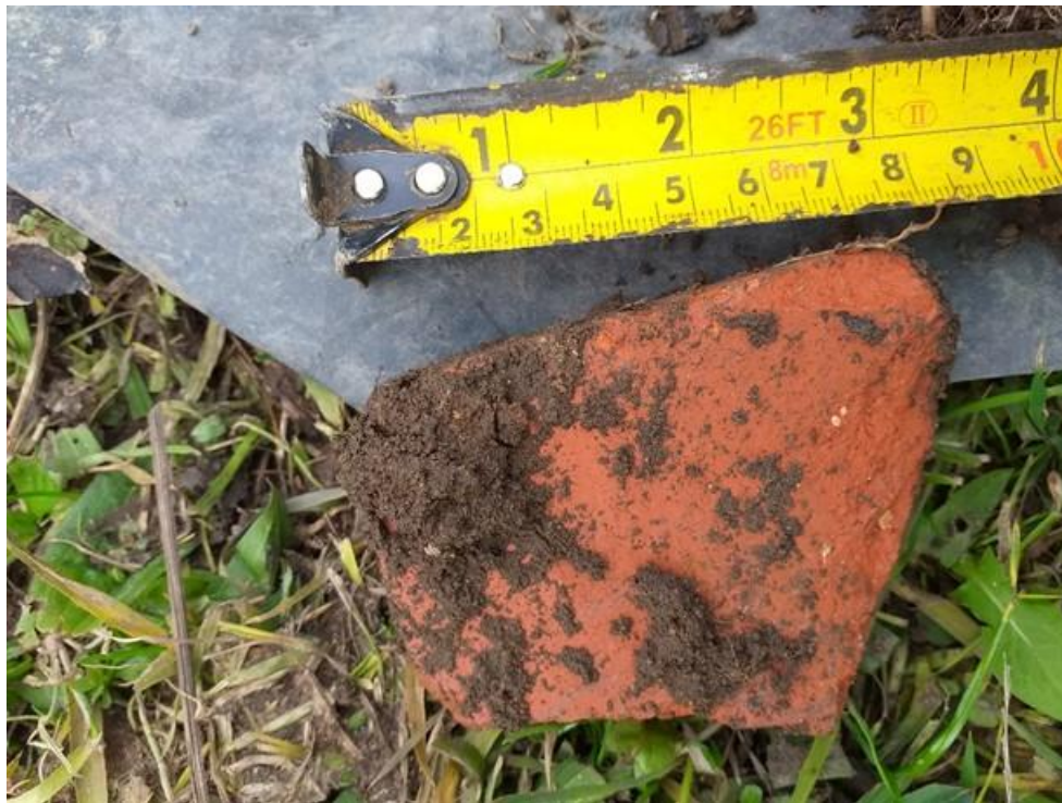
Photo 19: HP10 rare cobbles of brick in made ground (0.08 to 0.25mbgl).
