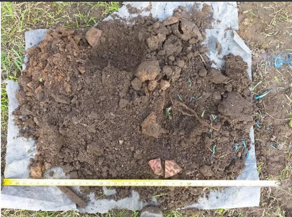
Photo 8: HP05 arisings recovered from 0 to 0.75mbgl. Depth below ground increases from right to left of image.
