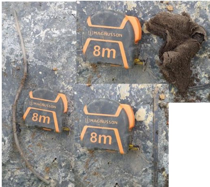
Photo 15: HP08 features of interest: left- 5mm diameter plastic tubing found near surface (0.05mbgl). In the made ground (0.07 to 0.4mbgl): top right- fabric, bottom right-metal bar.
