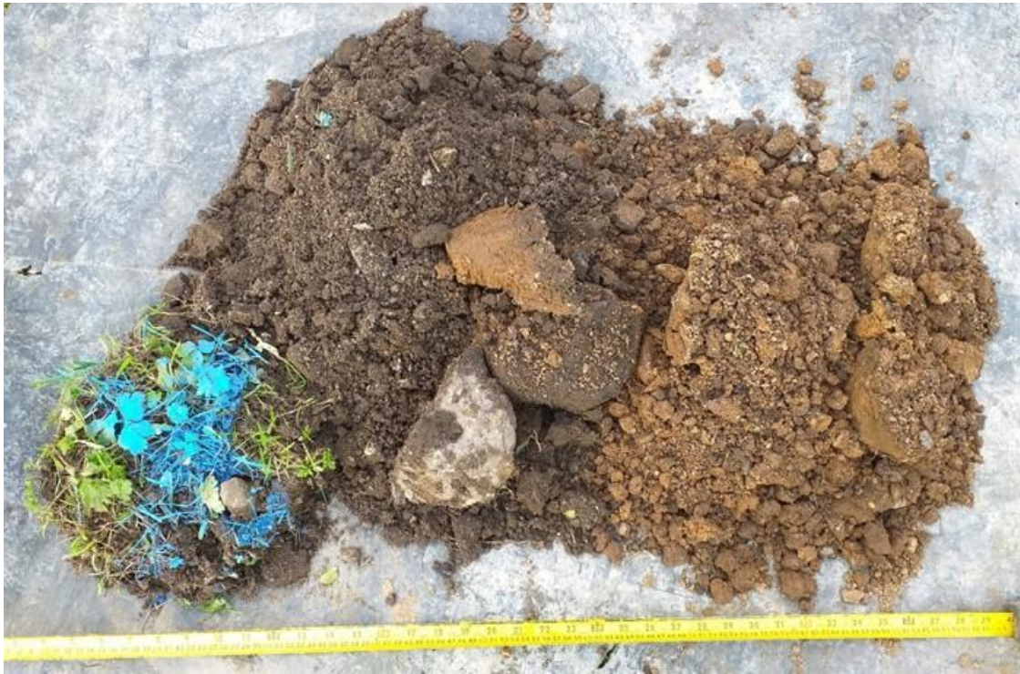
Photo 31: HP19 arisings recovered from 0 to 0.55mbgl. Depth below ground increases from left to right of image.
