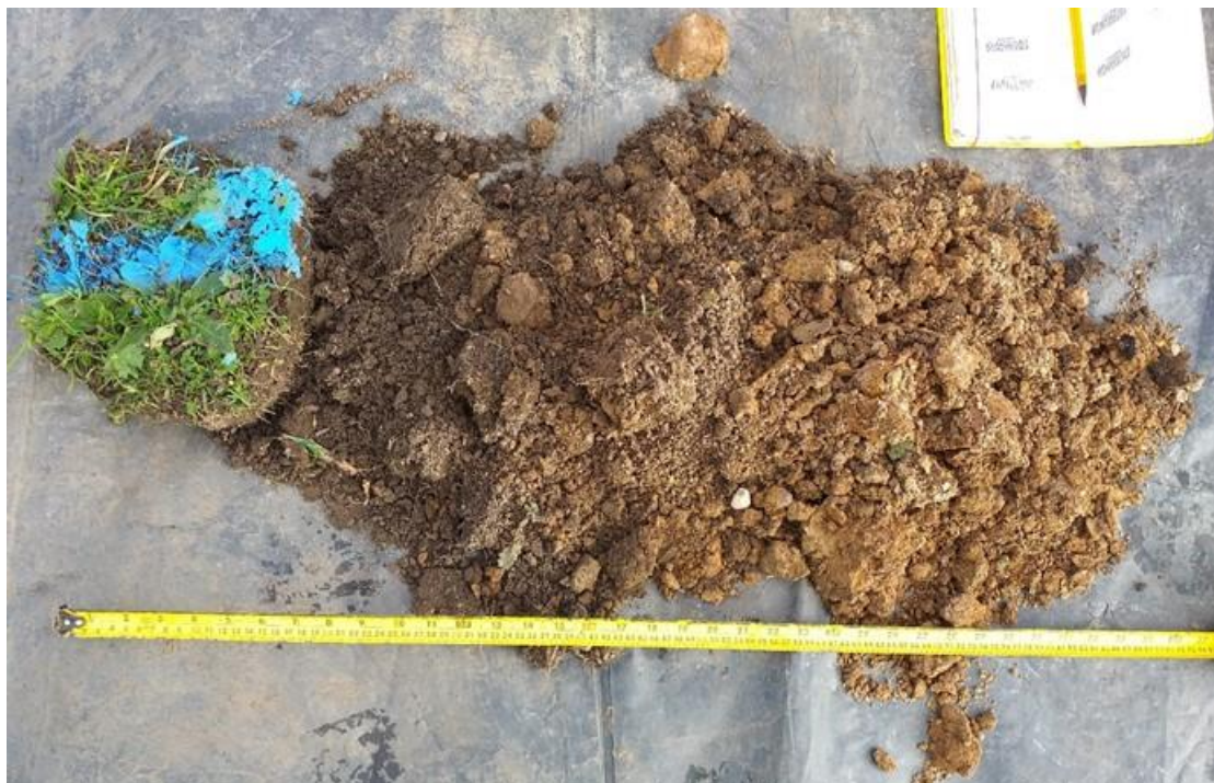
Photo 28: HP16 arisings recovered from 0 to 0.47mbgl. Depth below ground increases from left to right of image.
