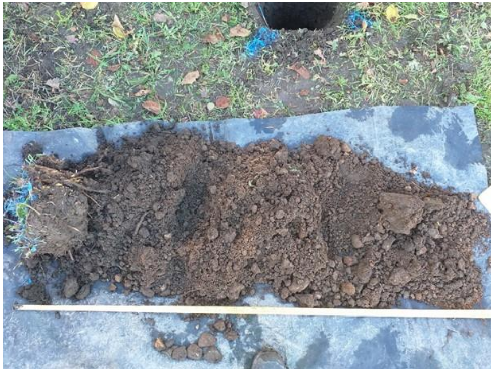
Photo 2: HP02 arisings recovered from 0 to 0.65mbgl. Depth below ground increases from left to right of image.
