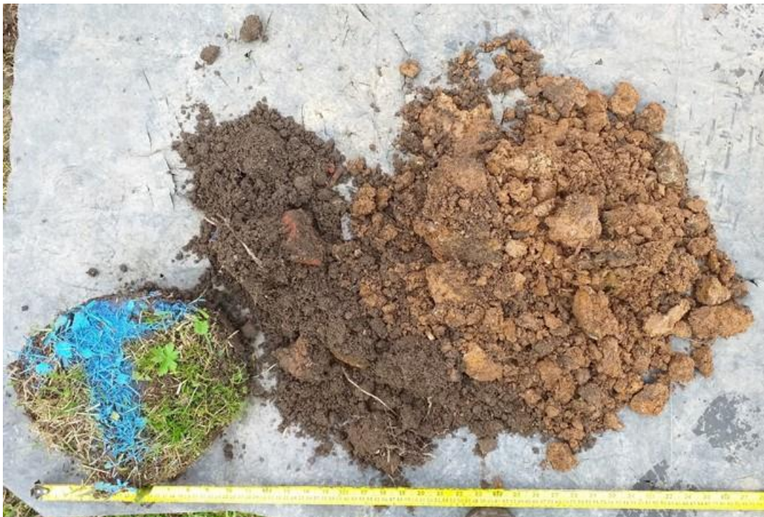
Photo 18: HP10 arisings recovered from 0 to 0.5mbgl. Depth below ground increases from left to right of image.
