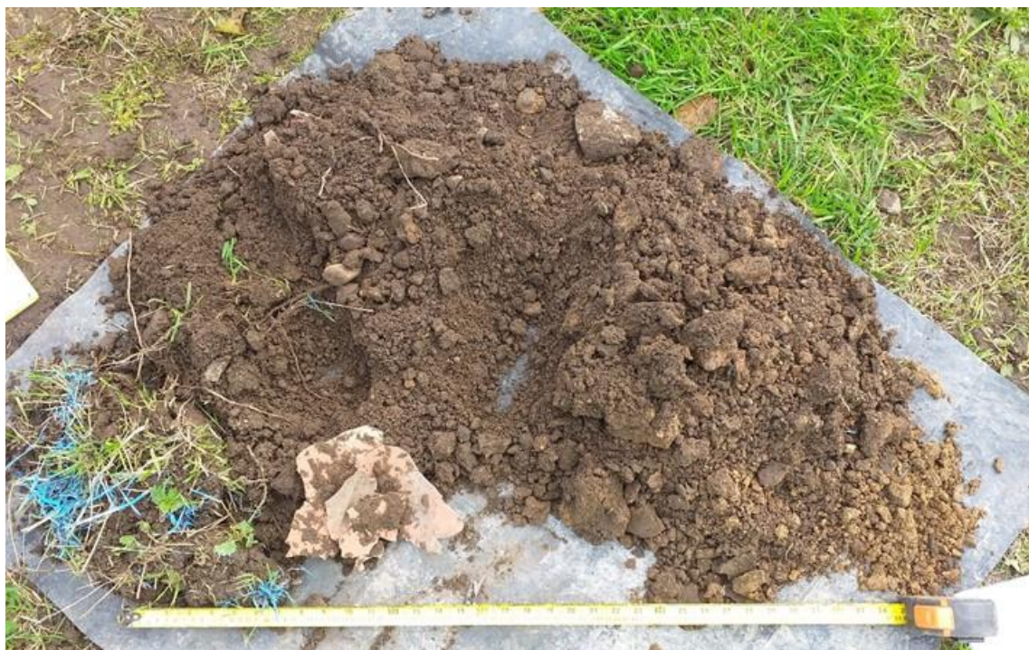
Photo 10: HP06 arisings recovered from 0 to 0.6mbgl. Depth below ground increases from left to right of the image.
