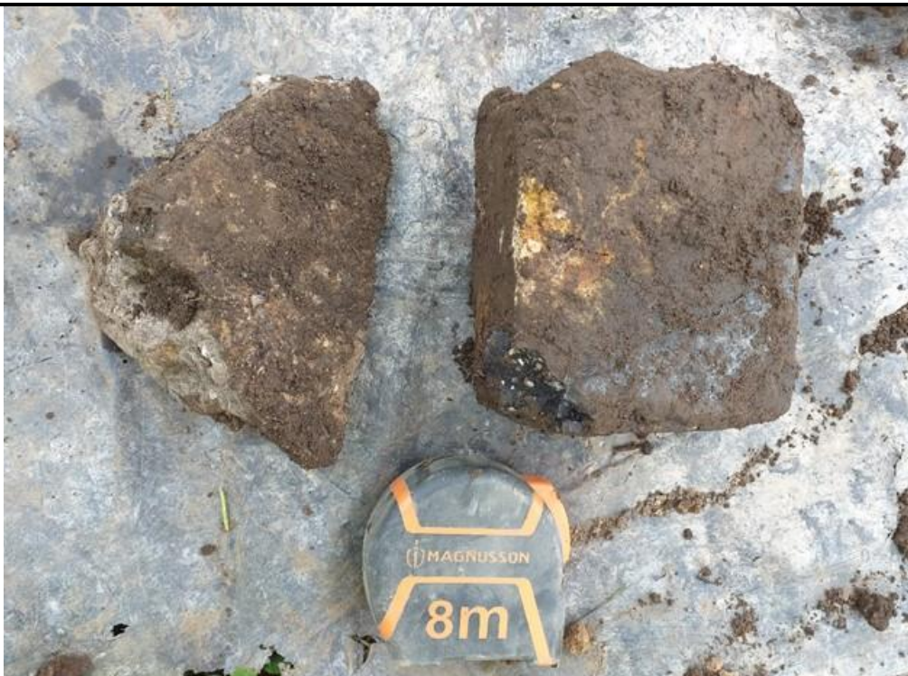
Photo 32: HP19 features of interest: rare cobbles of concrete (left) and brick (right) found in made ground (0.06 to 0.35mbgl).
