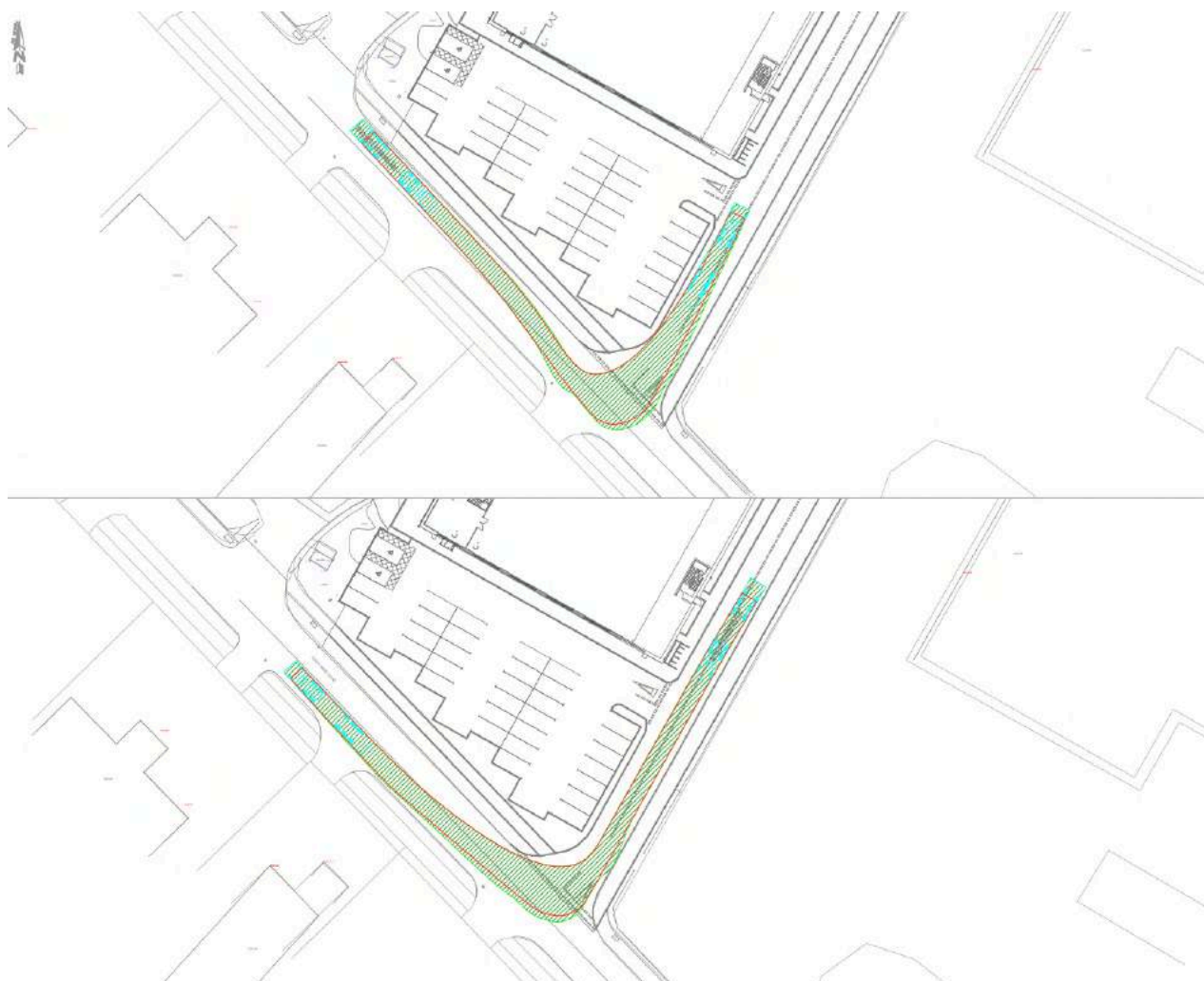
Figure 3.2 : Swept Path Analysis – Site Access Junction
