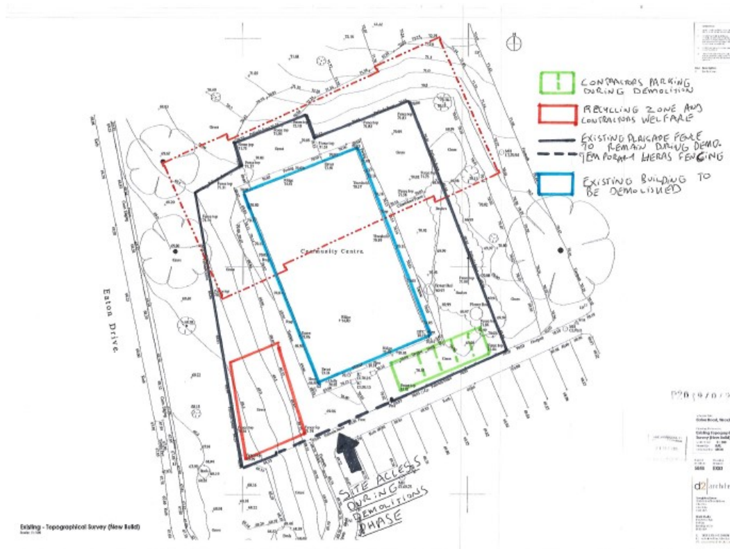
Site Set Up Plan During Demolition Phase
