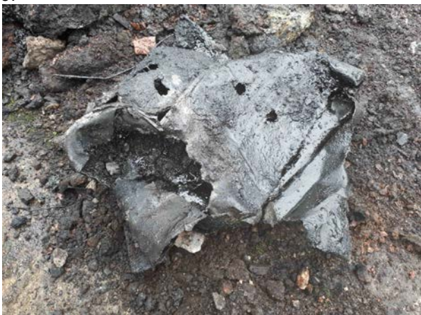
12.04.18 - Suspected contamination source following removal, an old oil drum with oily diesel residue within.
