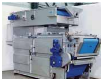
Belt Thickeners and Dewaterers
