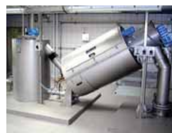
Drum Thickeners and Dewaterers
