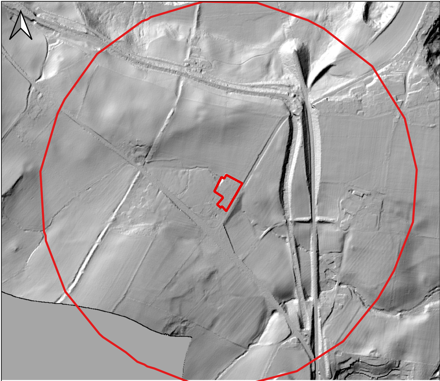
Figure 7. LiDAR 1m DTM – processed Hillshade.
