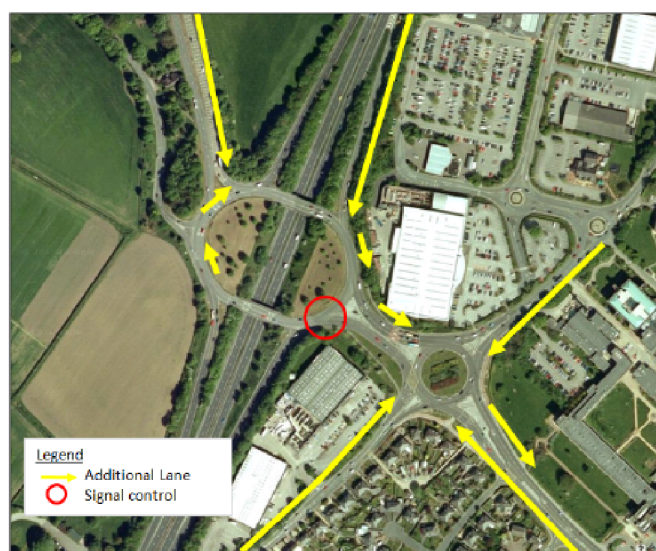
Figure 6.1 - Junction 5 High Level Improvement Measures
