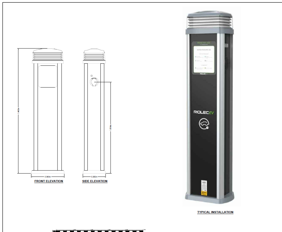
Figure 3.2: Electric Vehicle Charging Point Details
