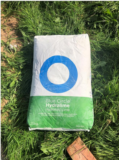
SAMPLE PANEL 02 - Handmade Cheshire Brick - Blue Circle Hydralime - Mix: 1 lime, 5 red sand 1 cement - Round Bar Pointing
