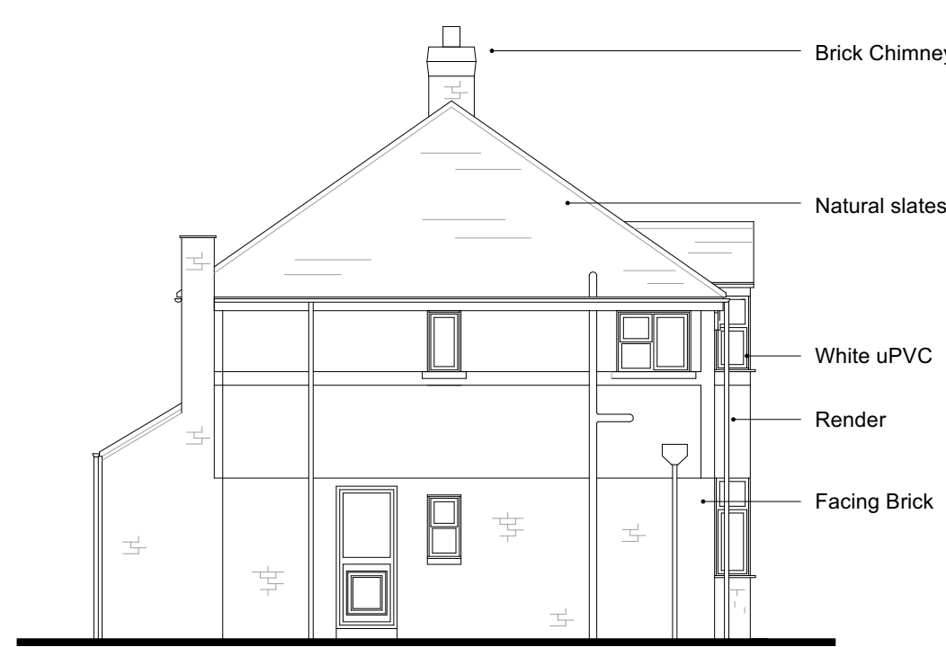
Existing Side Elevation View 'B' 1:100
