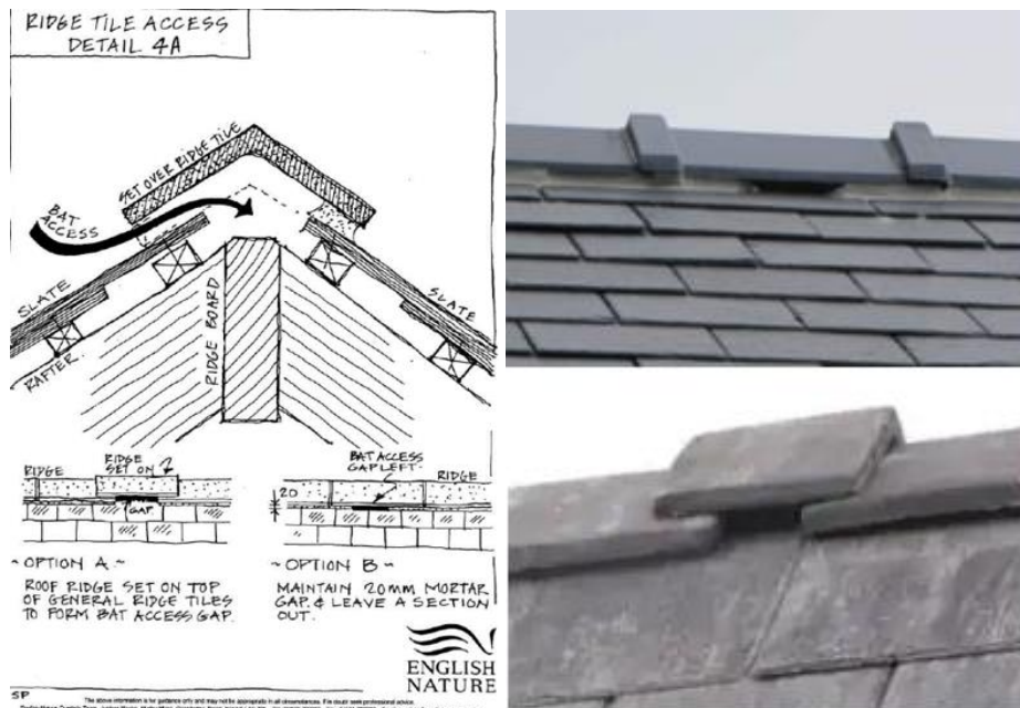
FIGURE 2.4: EXAMPLE OF RAISED RIDGE TILE ACCESS
