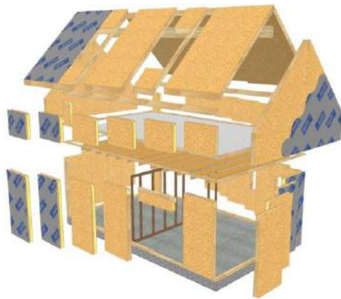
Typical SIPS Construction Illustration (Courtesy of Clays.com)
