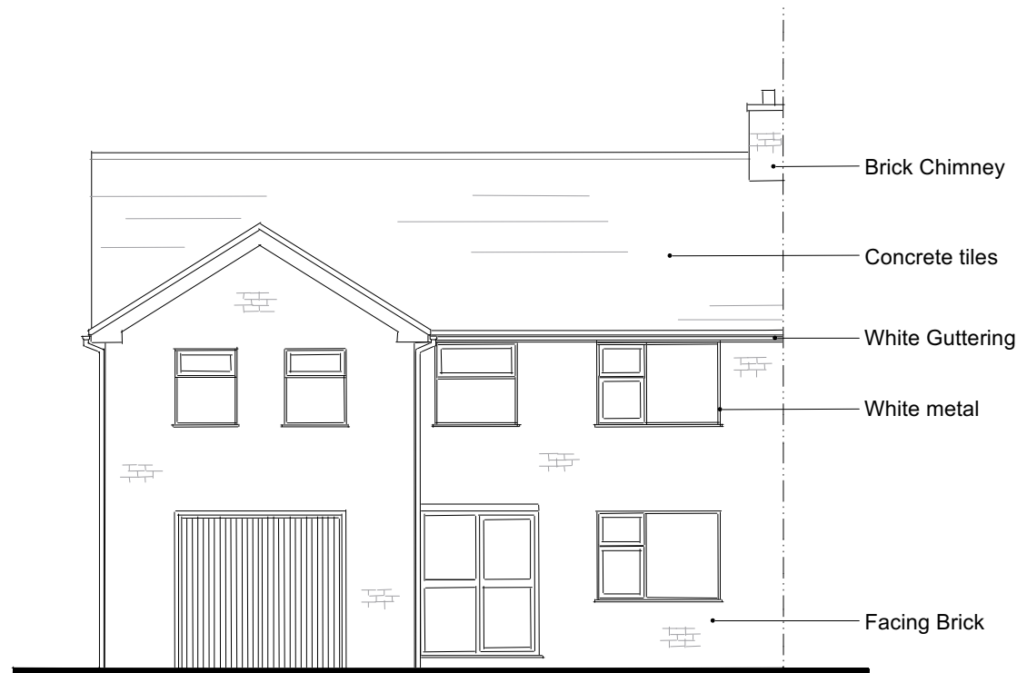
Existing Front Elevation View A - 1:100
