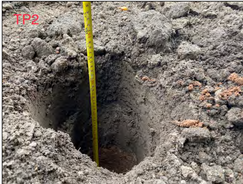
Plate 5 - Imported soil depth at TP2
