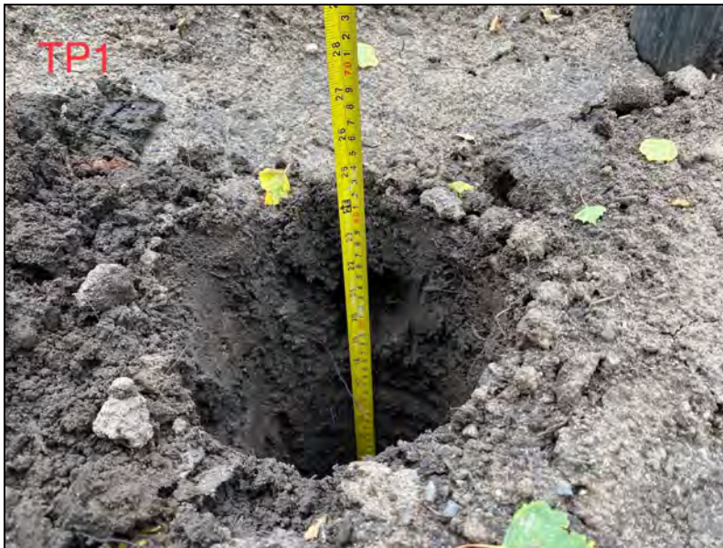
Plate 4 – Imported soil depth at TP1
