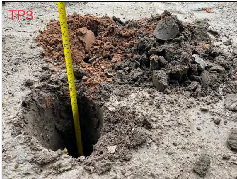
Plate 6 – Imported soil depth at TP3
