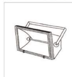
Type B: Floodlight/projector producing a fan-shaped beam
