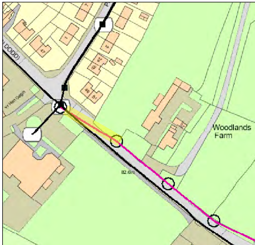
Fig. 8.04 - Existing BT overhead network requiring diversion
