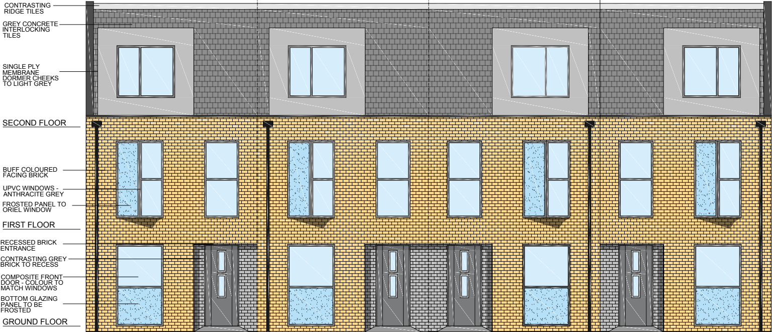
Proposed Front Elevation Scale [1:100]
