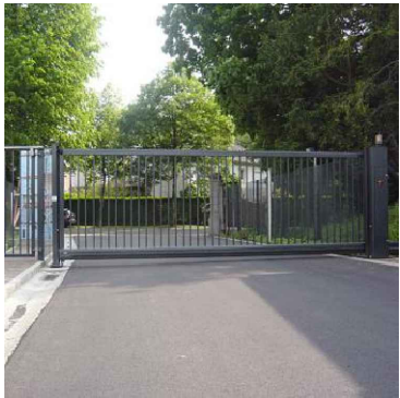
Typical example of proposed cantilever sliding gate. Colour RAL9005 Jet Black
