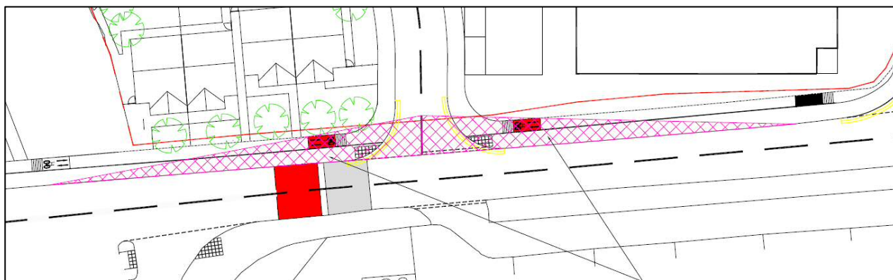
Figure 13: Proposed Llay New Road Access Visibility Splay
