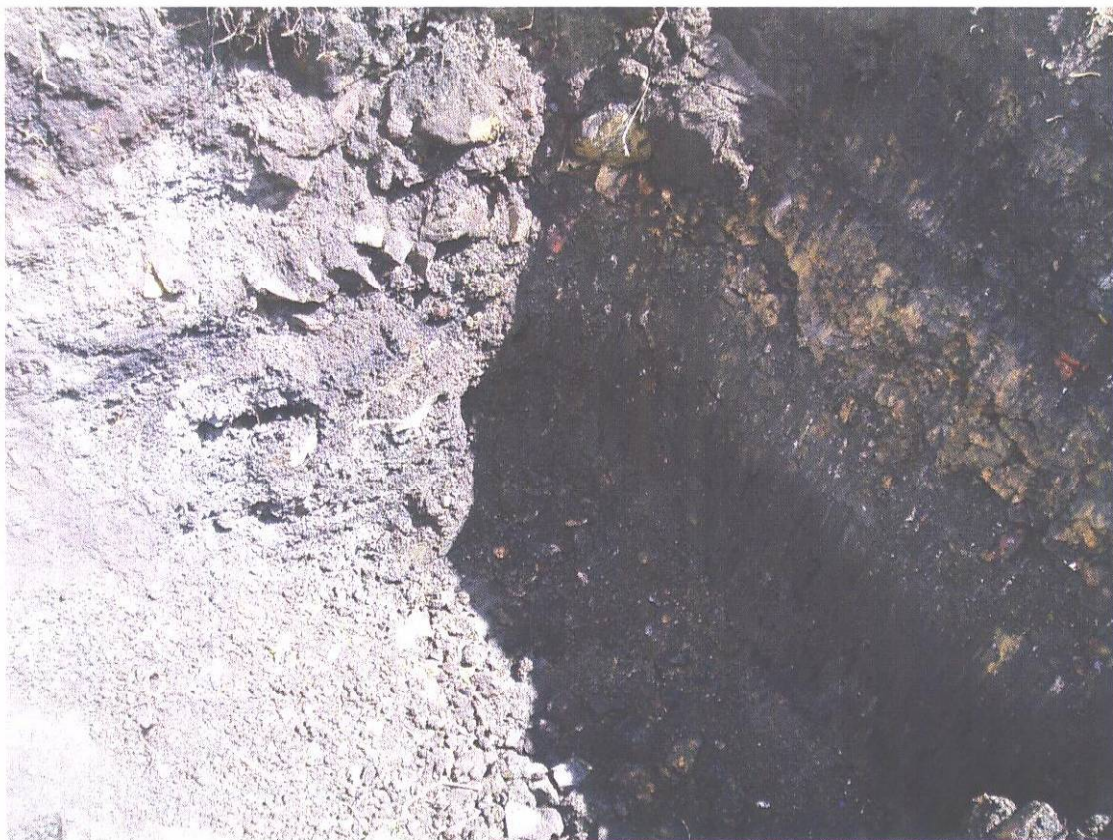
Made ground extending beneath railway embankment construction in far corner of pit.
