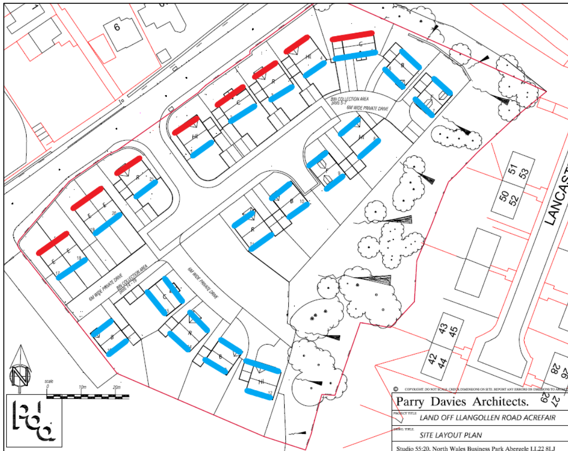
Figure 4.1 - Site layout showing recommended glazing types
