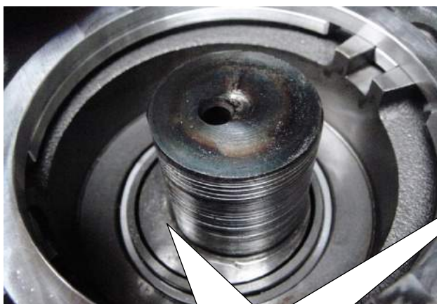
The crankshaft is worn.
