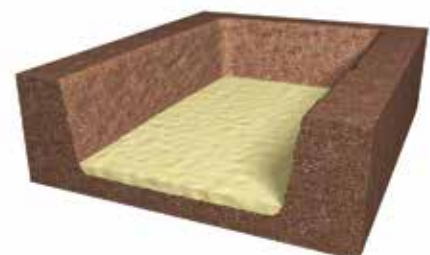
Step 2 - Lay sub-base.
