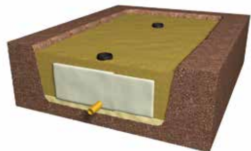
Step 8 - Lateral backfilling.
