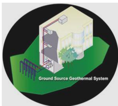
Ground Source Heat Pump Installation
