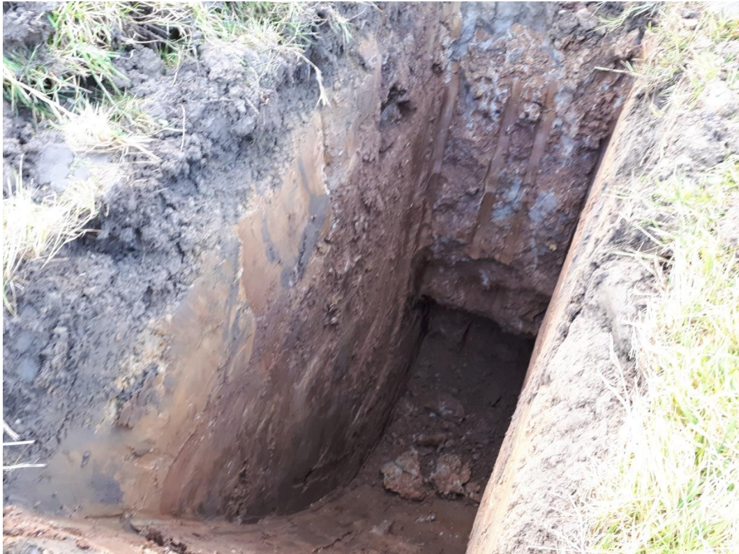
Trial Pit 01 – Pit Walls
