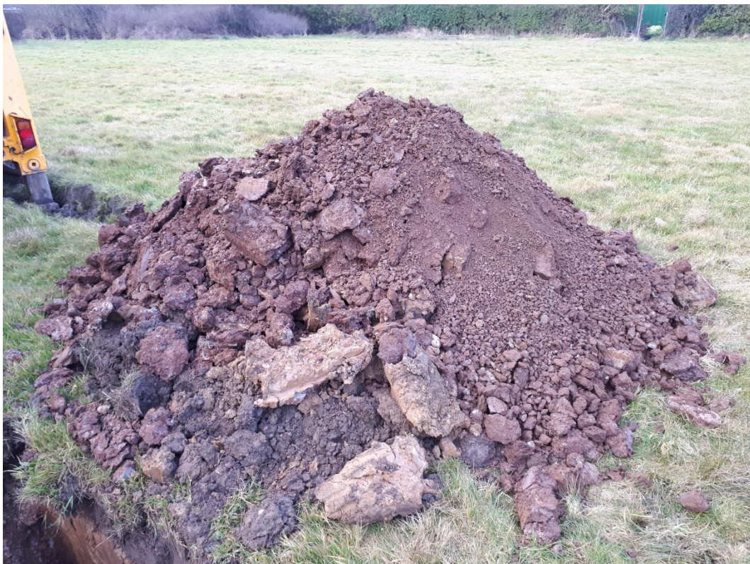
Trial Pit 01 - Arisings
