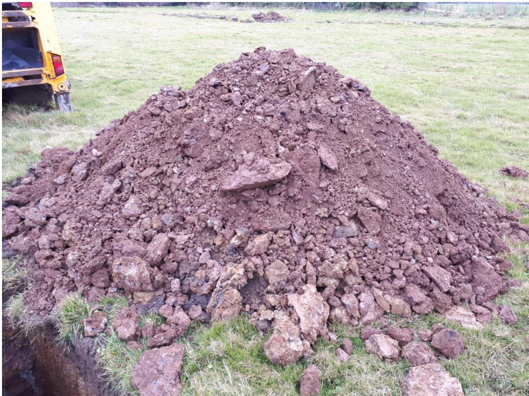
Trial Pit 04 - Arisings
