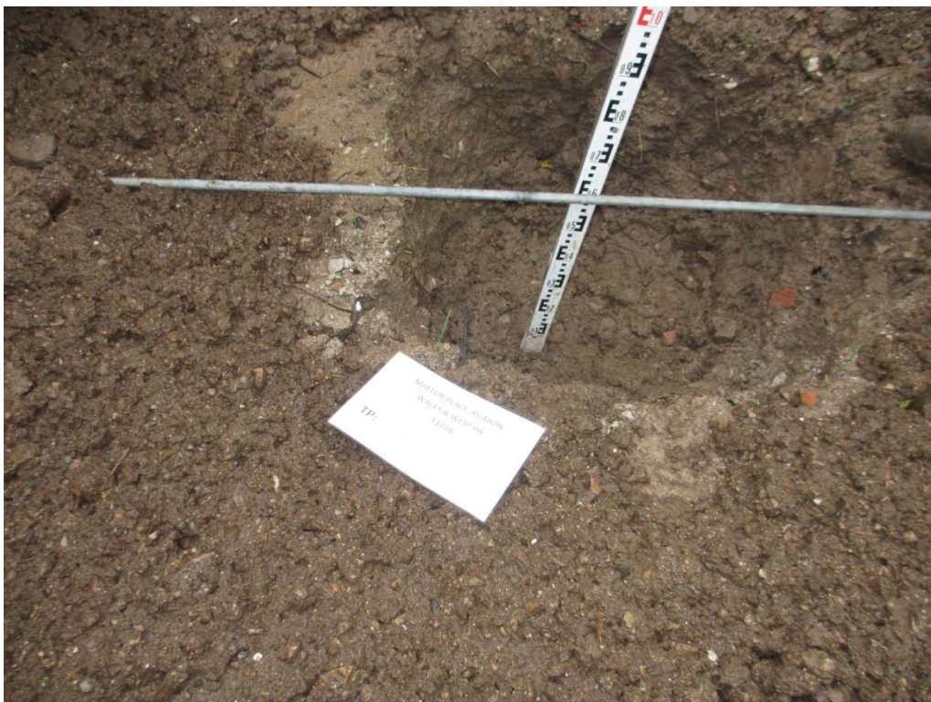
Photo 4 – Plot showing capping thickness >0.60\text{m} at Plot 10
