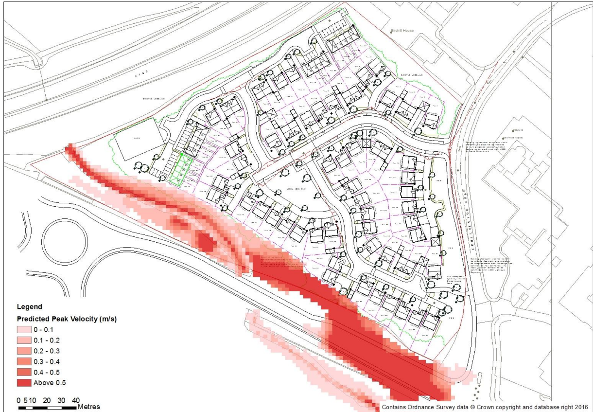
Figure 5 – Flood Velocity Information for the updated 100% blockage during the 1% AEP event plus climate change
