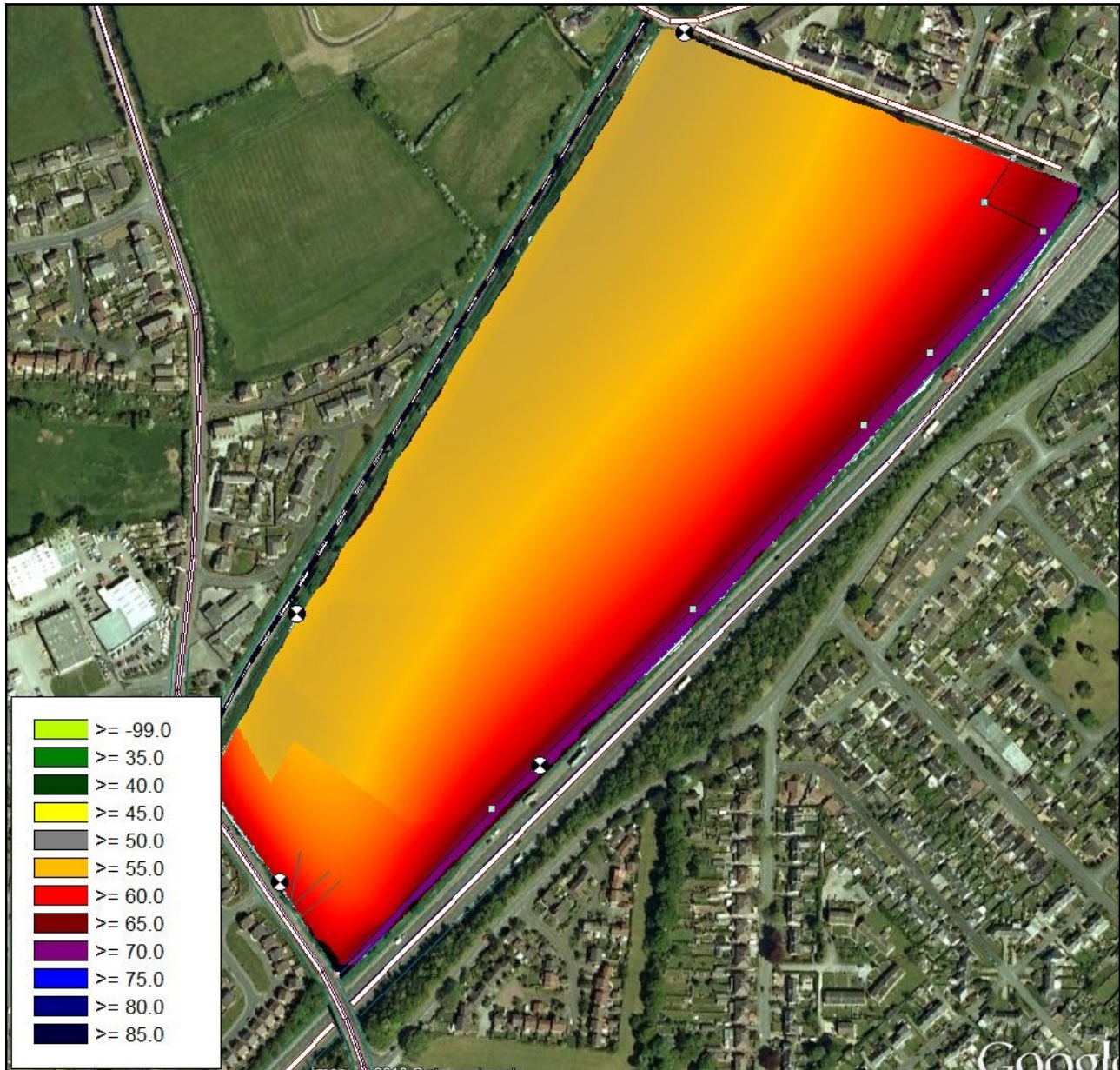
Figure 6.7: CadnaA View Showing Predicted Night Time L_{Aeq} Noise Propagation Across the Site at 4m Height - With 2m Barrier
