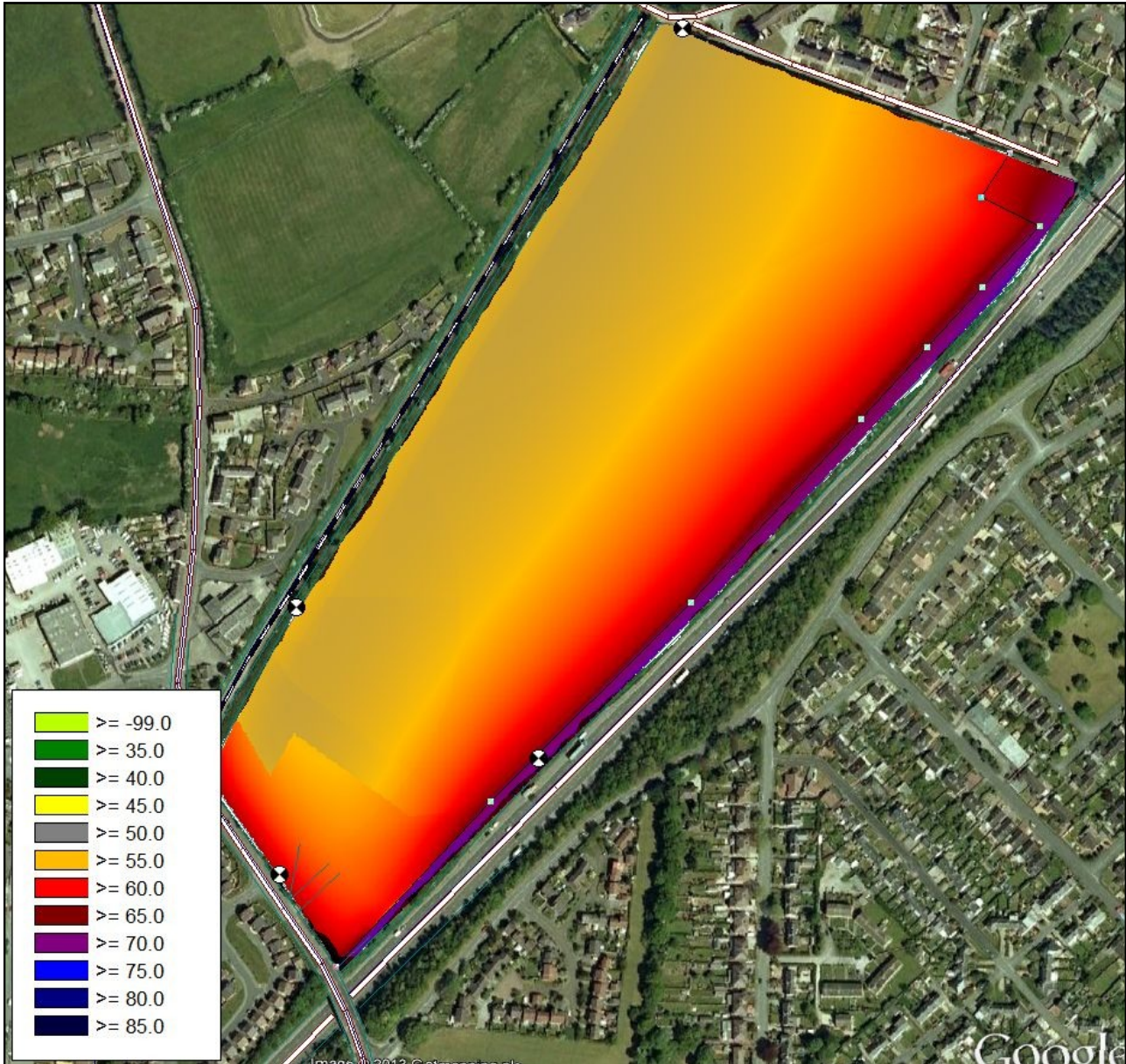
Figure 6.11: CadnaA View Showing Predicted Night Time L_{Aeq} Noise Propagation Across the Site at 4m Height - With 3m Barrier
