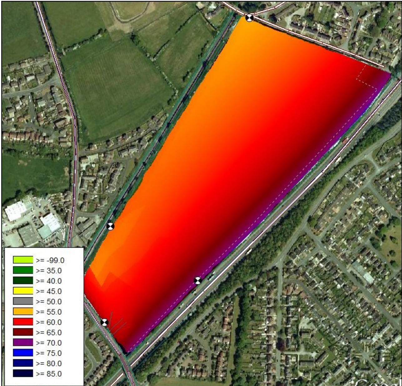
Figure 6.3: CadnaA View Showing Predicted Night Time L_{Aeq} Noise Propagation Across the Site at 4m Height
