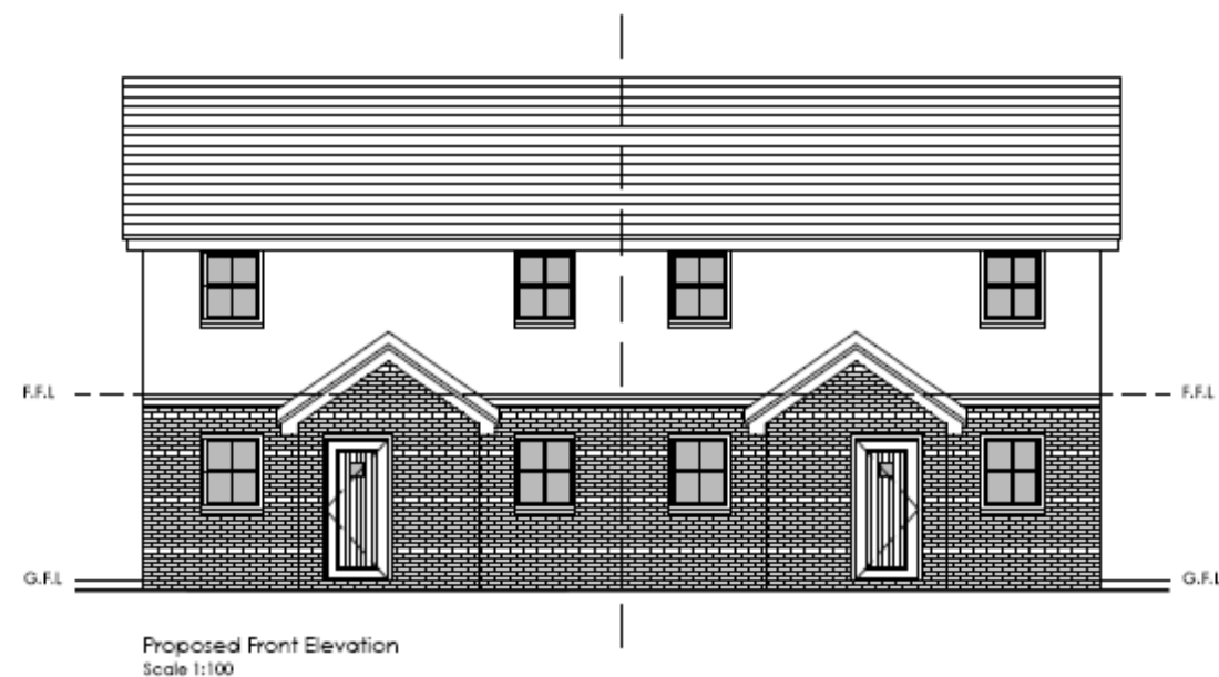
Fig n) Elevations (White Render & Facing Brick)
