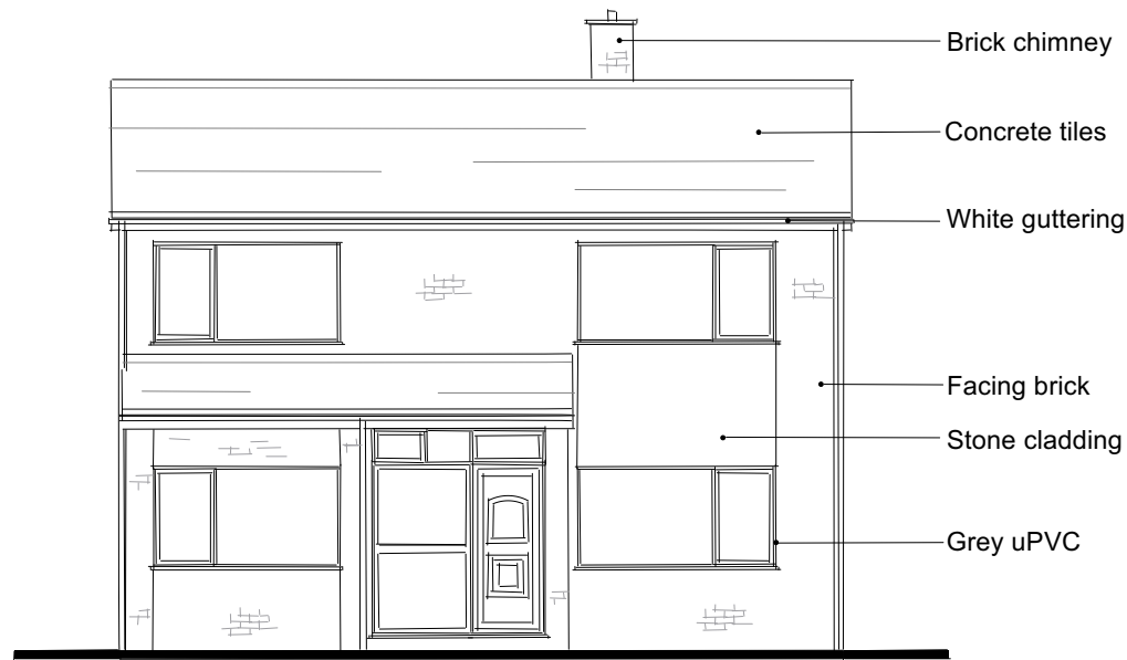
Existing Front Elevation View A - 1:100
