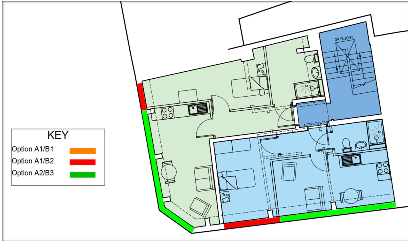
Figure C 2: Third floor glazing and ventilation mark-up's
