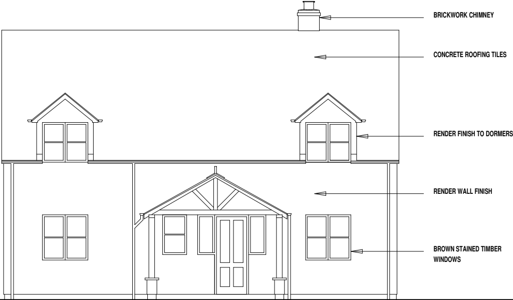
EXISTING FRONT ELEVATION
