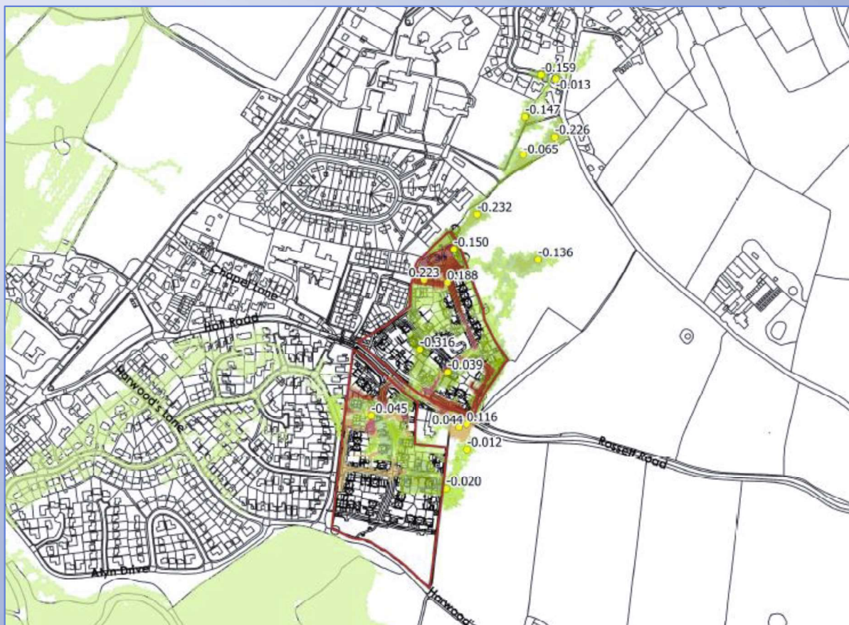
Figure 6: 0.1% AEP with blockage – Depth Difference Plan (Betts Hydro, 2021)
