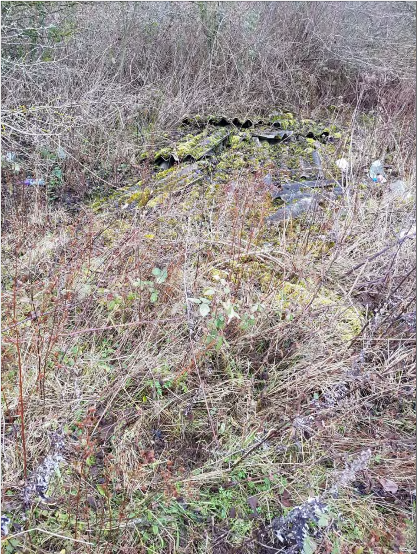
Photograph 2: Fly tipped cemented asbestos sheeting immediately next to the eastern access track.
